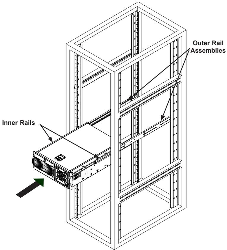
**Figure 3: Mounting the Chassis into a Rack**
