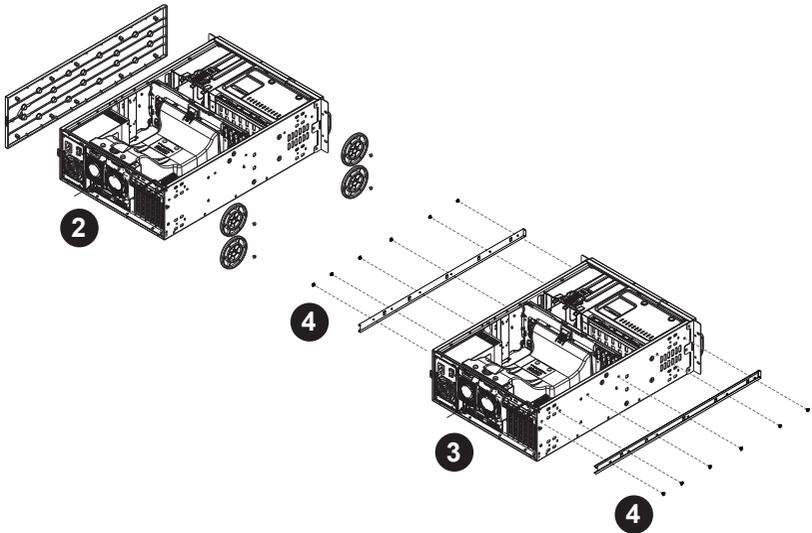
**Figure 1: Installing the Inner Chassis Rails**
